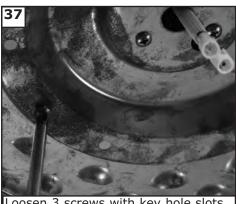
Loosen 3 screws with key hole slots.
